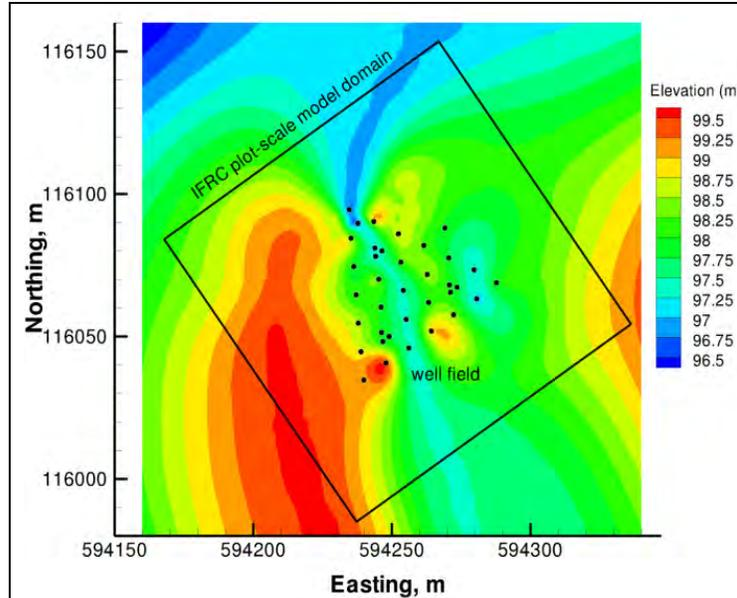
**Figure 3.** Map showing interpreted elevation of surface of Hanford-Ringold Fm contact in vicinity of Hanford 300 Area IFRC site. Black dots show well locations and black square shows approximate plan-view extent and orientation of numerical flow and transport models being applied to evaluate field experiments. Note apparent channel feature extending through center of well field.
