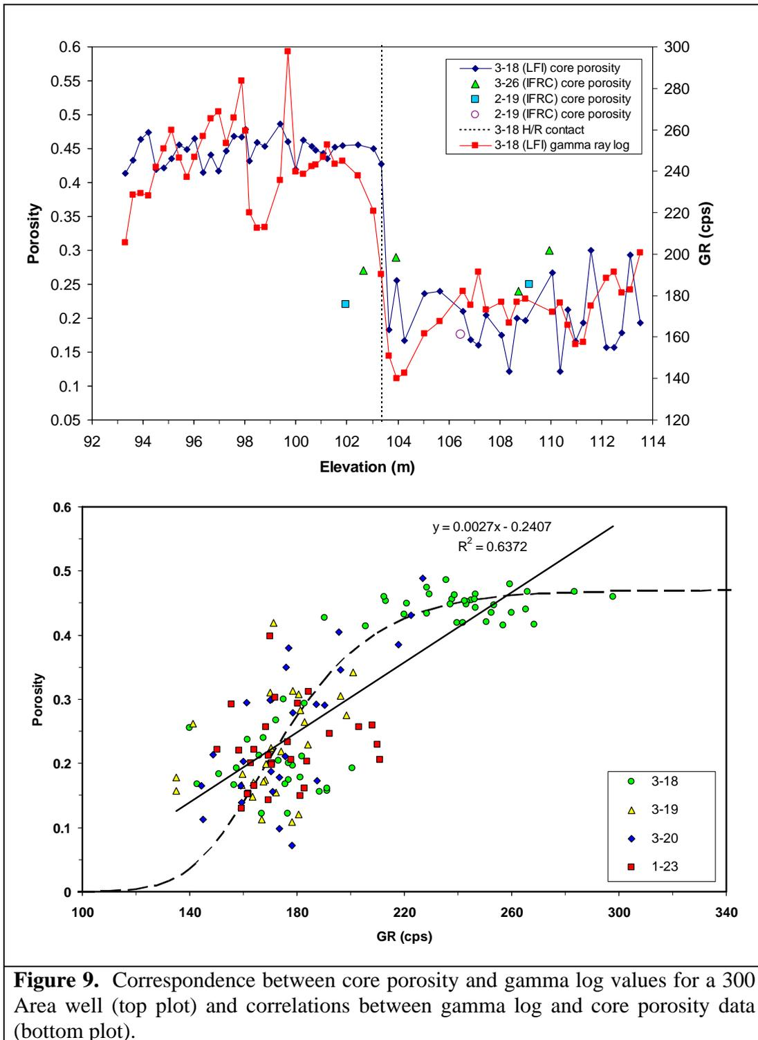
**Figure 9.** Correspondence between core porosity and gamma log values for a 300 Area well (top plot) and correlations between gamma log and core porosity data (bottom plot).
