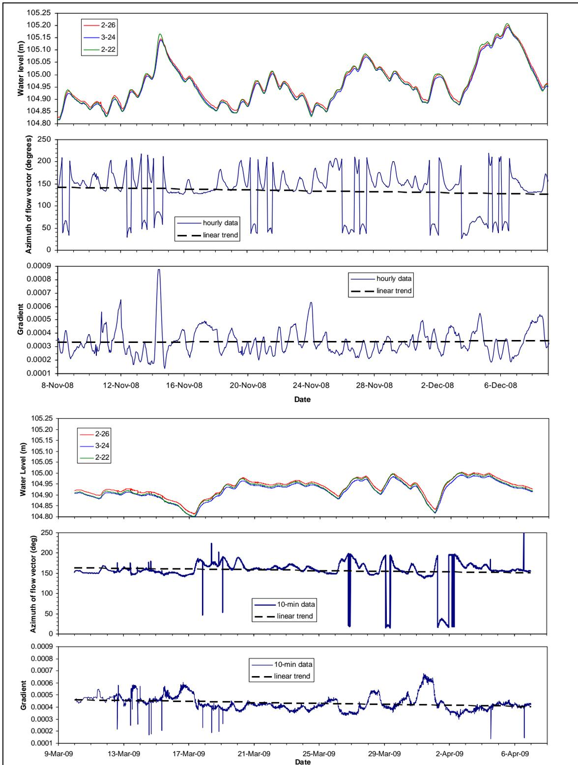
**Figure 7.** Observed water levels and computed flow directions and gradients during the November 2008 (top 3 panels) and March 2009 tracer tests (bottom 3 panels) at the Hanford 300 Area IFRC site. Note that the flow conditions were much more stable during the March 2009 test.
