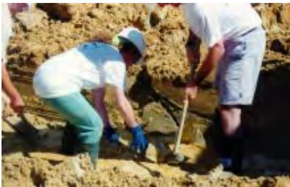
**Figure 10.** Collection of Horizontal Intact Cores from Below the Water Table (saturated zone) During the Excavation in the Narrow Channel Focus Area in August 1998. The excavator was used to create a smooth surface below the water table and aluminum Shelby tubes were driven into the face of the excavation in the orientation of local groundwater flow. These intact cores will be used for transport studies that will be used to design the field bacterial transport experiments.
